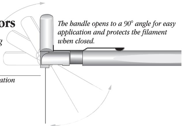
The handle opens to a 90° angle for easy application and protects the filament when closed.
